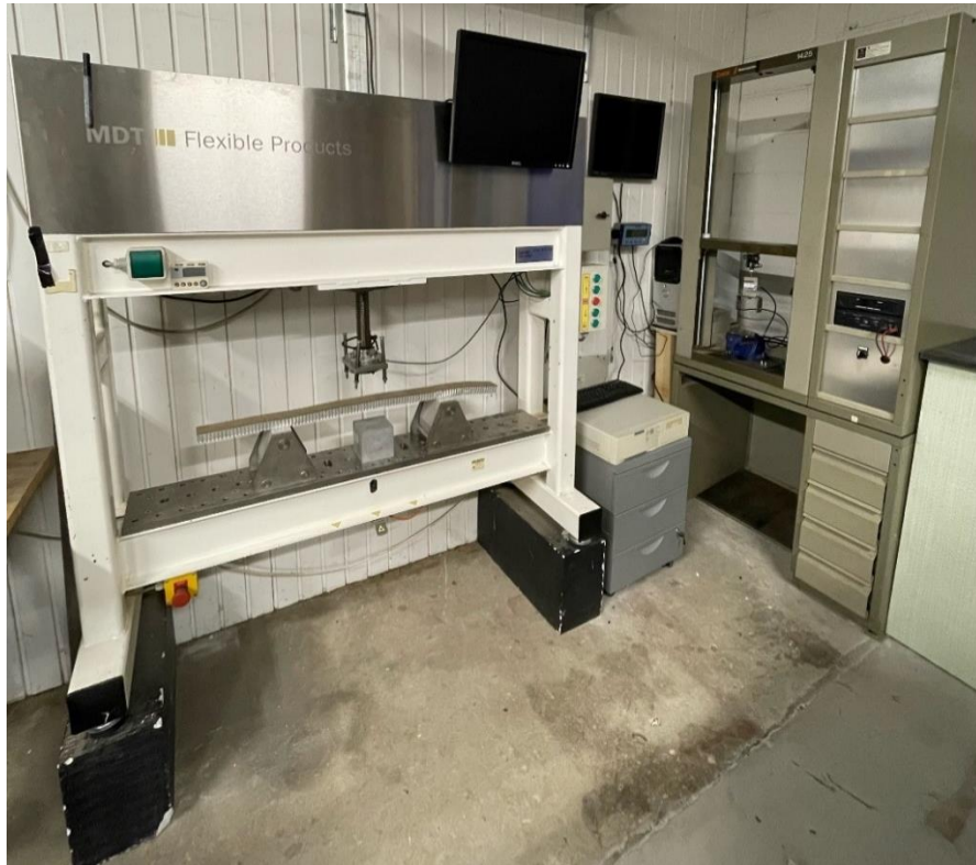
Figure 1: Static mechanical tests provided at MDT A/S: Bending test 3-4 points (shown in the left side of the image) and tensile test (shown in the right side of the image)
